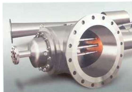
Multiple-nozzle assembly viewed through the suction connection.
