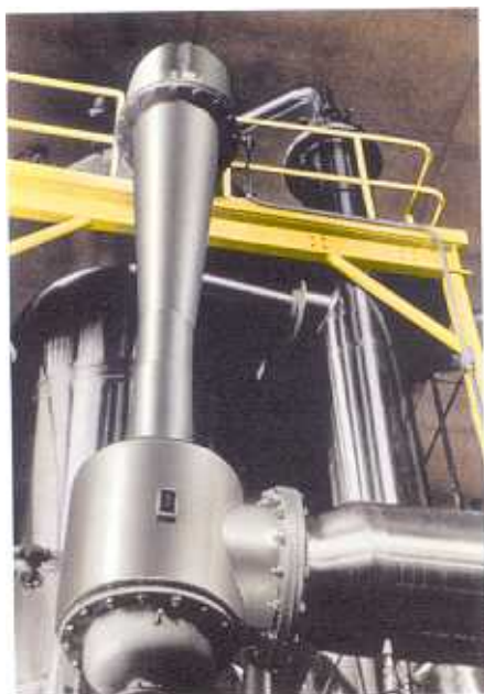
This triple-effect, falling-film, dairy products evaporator produces as much as 150,000 gallons of condensed milk per hour. A thermocompressor between the first and second effects reduces steam consumption. As a result, the evaporator uses less water and requires less heat transfer area.
