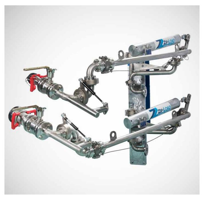
This type of loading arm is especially designed to transfer liquids and gases where vapour return is necessary. It is suitable for the bottom loading/unloading of road or rail tankers with flange connections or via a coupling. The loading arm has a long reach and is suitable for applications where the tanker connection flange cannot be accurately positioned
