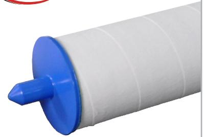
The PEACH Gemini, Series PGC, cartridge is specifically designed for use with the PEACH Gemini PuraSep vessel in natural gas filter-coalescing applications. Its unique patented design provides dual flow path filtration with all the added benefits of PEACH technology. Gas flows outside-to-inside through the 1st Stage of the cartridge where
