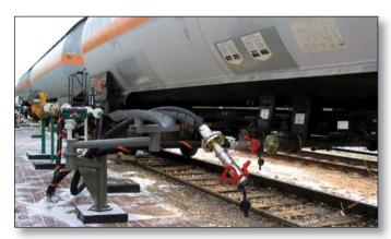
TODO-GAS® DRY-BREAK® couplings are designed specially for the safe an efficient handling of LPG in both liquid and vapour phases. Certified towards European Directive 97/23/EC (P.E.D.) category II.
