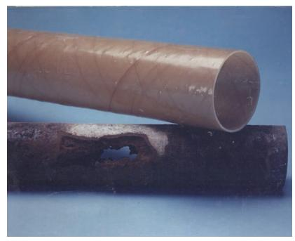
Fiberglass has a long corrosion-free service life and requires no coating or cathodic protection.
