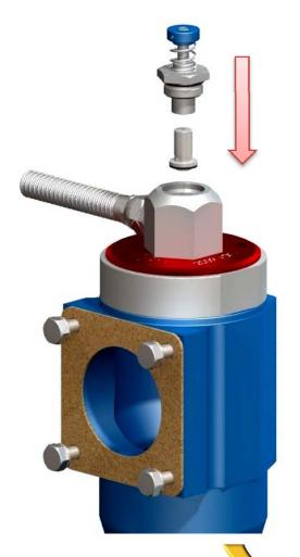
Replace the white poppet and hexagonal cap with non-spark spanners (11/4 and 11/2 inch AF).
