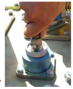
Whilst holding the top down a mild 'thump' and fill hose reaction should be noticed indicating that the shut off valve has closed.
