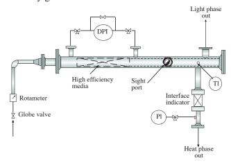
The testing units are fully operational, selfcontained packages, consisting of pressure vessels (certified to such local codes as ASME, Stoomwezen, Codap and Ad-Merkblatt) with sight glasses to observe performance, instrumentation and piping.
