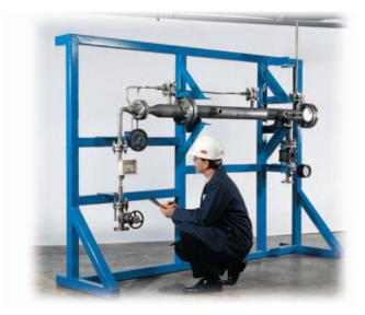
Measurements of pressure drop, flow rates, and separation efficiency may be taken by the customer or experienced KOCH-OTTO YORK<sup>®</sup> engineers. The collected data give the best possible understanding for the tested stream, including the effects of contaminants, the potential for fouling or corrosion, and any other unforeseen complications. Performance guarantees to duplicate test unit performance are routinely given.
