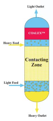
In vertical vessels, such as counter-current flow solvent extractors or wash columns, it has been common industry practice to install a horizontal flow coalescer in a separate, external vessel. By installation of a COALEX<sup>TM</sup> liquid-liquid separator within the extraction/wash column, as shown above, a separate vessel, with its instrumentation, plot plan space, foundations and installation costs, is eliminated.
