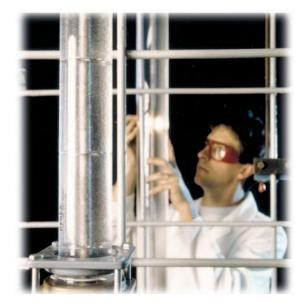
Since small uncertainties can still exist, because of possible changes in the emulsion during shipping and storage, the most reliable design data will always be obtained by onsite slipstream testing at actual process conditions.
