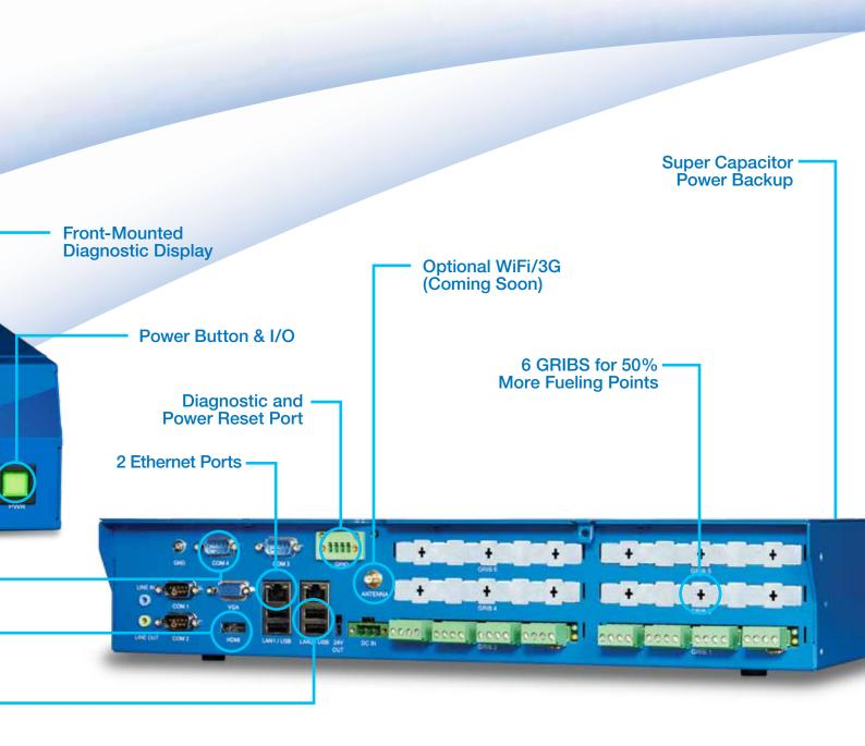
The newest generation of the Fusion forecourt system is configured for easier accessibility and serviceability. With the power button, I/O, and USB ports on the front, running the system and pulling data information is quicker and easier. The front-mounted display allows you to see alerts and diagnostic information clearly. Add in the fact that there are no moving parts behind the face, and you've got a robust and hardened solution to address your current needs and adapt as those needs evolve.
