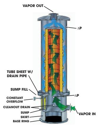
Figure 4. FLEXIFIBER  $^{\circ}$  mist eliminator for lube oil tank vents on gas or steam turbines.
