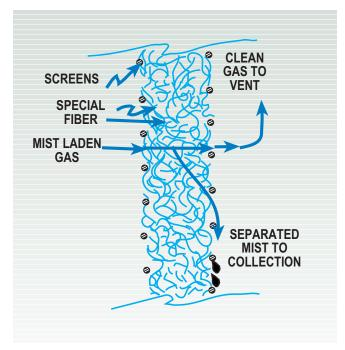
Figure 1. Single stage vertical FLEXIFIBER® mist eliminator
