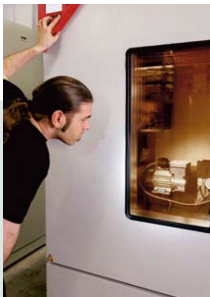
climatic exposure test cabinet – tests to extreme conditions.
